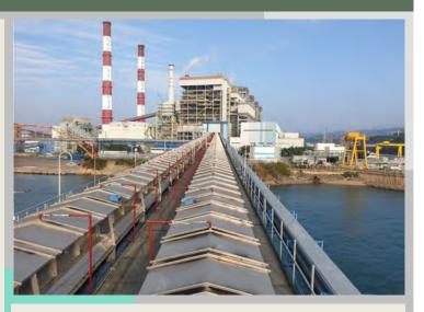
Because there are no idlers, common maintenance associated with a conventional conveyor is eliminated. The **Grisley ASC** operates with only four bearings - two at the head pulley and two at the tail. **Grisley ASC's** standard design includes an air-supported return plenum, so there are no idlers or bearings on the return side of the conveyor.
