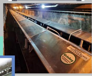
The Retrofit Plenum provides easy dust collection in tight spaces such as tunnels or areas well above grade with no additional ducting needed. The dust-tight design adds significant increase in safety to the work area environment.
